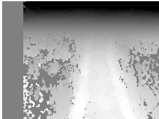
Figure 4.6 An example of a height map, H . Darker pixels are further from the assumed ground plane.
