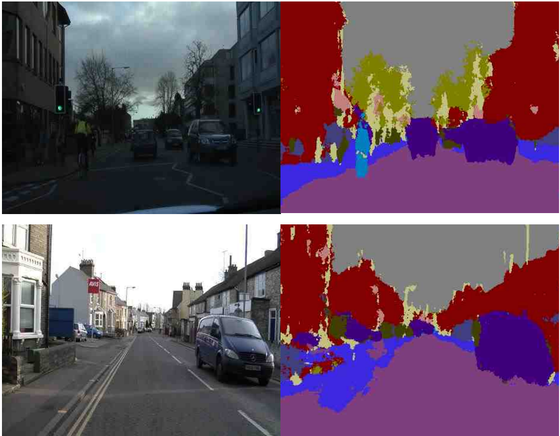
Figure 3.3 Example images from the Camvid data set along with corresponding Segnet output with each pixel assigned one of eleven class labels: road (dark pink), vehicles (dark purple), pavement (light blue), buildings (red), sky (grey), poles (yellow), trees (light gold), cyclist (turquoise), road signs (light pink), fence (dark blue), pedestrian (dark gold).
