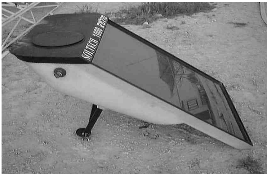
Figure 2.9f An Integrated collector–storage system [60].
