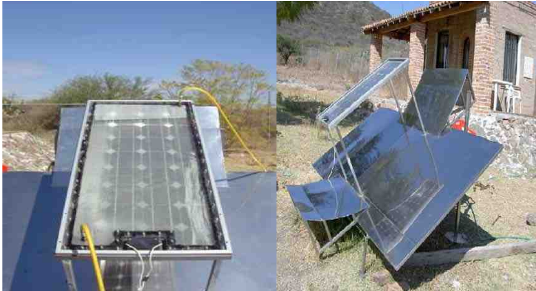
Figure 2.9k A bifacial PV module [69].
