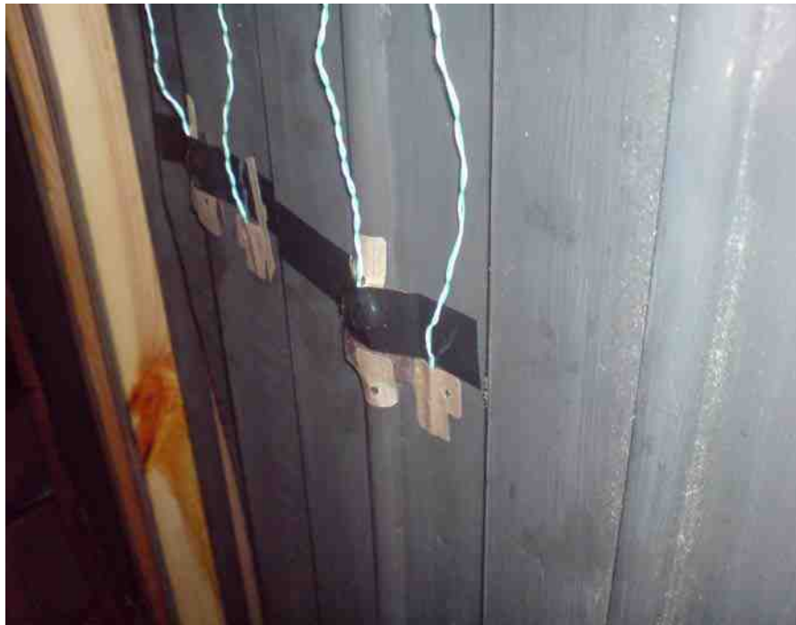
Figure 6.4j Surface temperature measurements setup.
