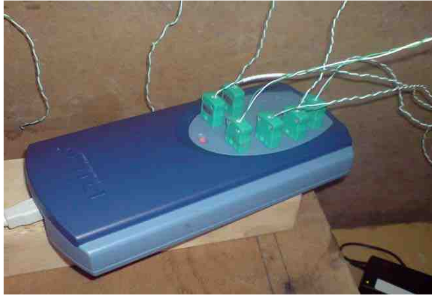
Figure 6.2h Data logger with thermocouples attached.
