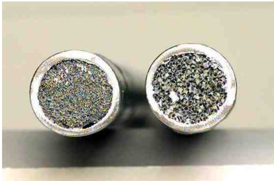
Figure 3.6e Metal-foam filled tubes [82].
