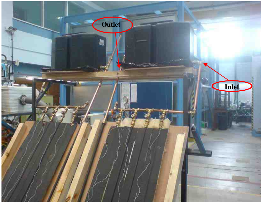
Figure 6.4b Water tanks connected to the collectors.
