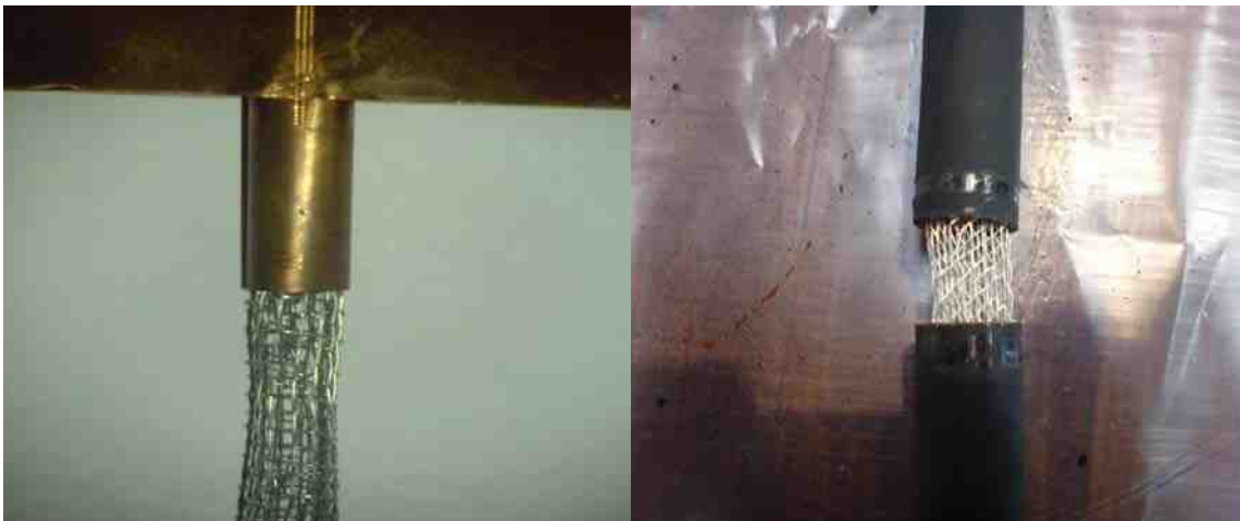
Figure 6.2e Porous medium inserted in a copper pipe.
