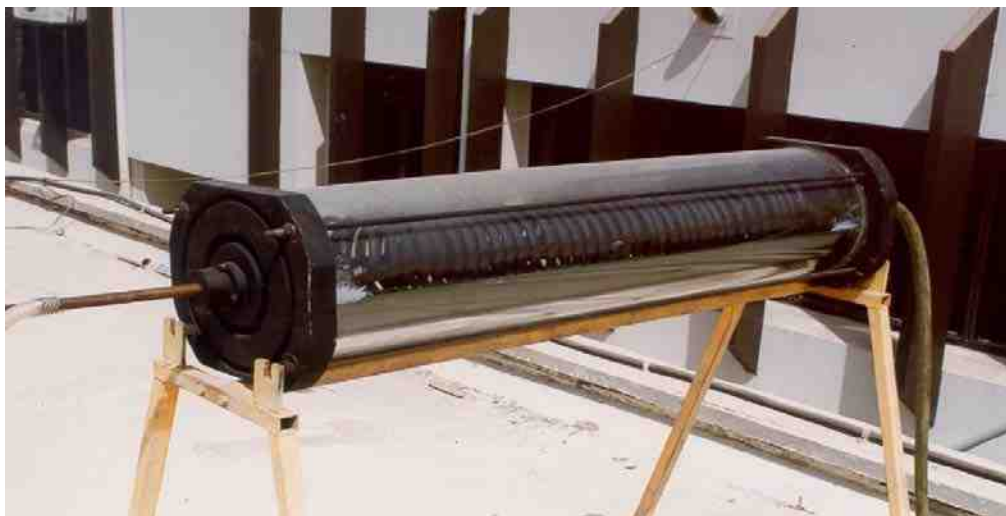
Figure 2.9i A cylindrical solar water heater [63].
