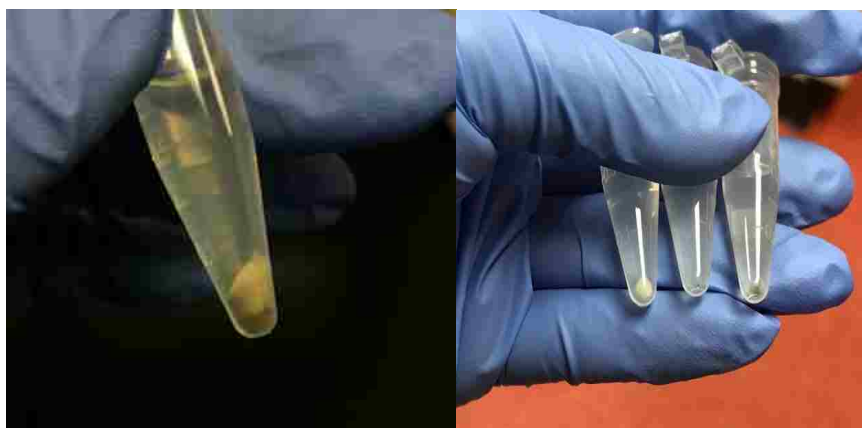
Figure 12. Micro-centrifuge tubes showing the two layers formed upon settling of bacterial cells on top of AgNPs (left), and (right) the isolation of cell precipitate separately from AgNPs.
