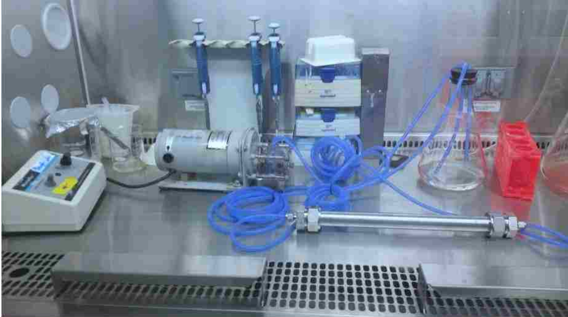
Figure 3: Example of a Simple Hollow Fiber Membrane Bioreactor
