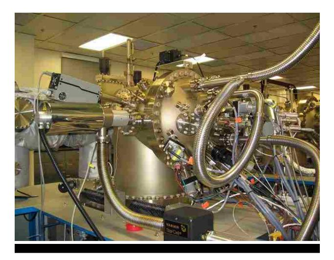
The degas chamber is equipped with a heater so that samples can be degassed to remove water molecules and other organic contaminations before loading to the growth chamber. Both the load-lock and degas chambers are pumped down by turbomolecular pumps while both the transfer chamber and growth chamber are pumped down by a detachable turbomolecular pump only at the beginning, and vacuum is kept by ion pumps and titanium sublimation pumps.
