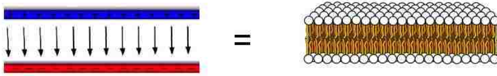
Figure E.1: Bilayer lipid membrane is considered as a Parallel plate capacitor
