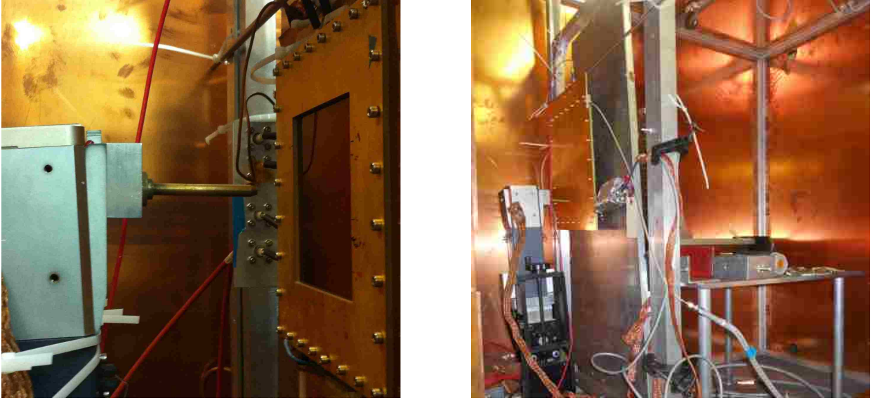
Figure 5.2: Left: Collimator positioned normal to the GEM surface. Right: GEM mounted inside a Faraday cage [25].
