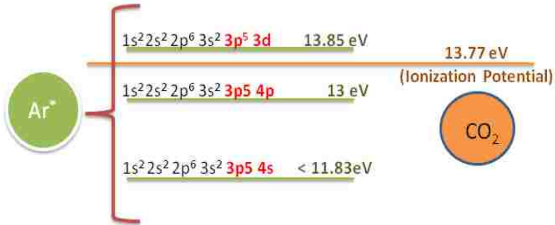
Figure 3.1: Excitation levels of Ar atom in comparison with the ionization potential of CO 2
