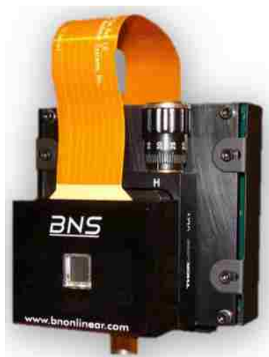
Figure 3.7: A photograph of the BNS phase-only spatial light modulator (SLM) from the BNS user manual. A device used to modulate the phase of incoming light which is then reflected.
