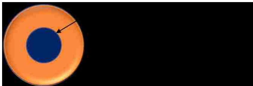
Figure 3 A cross-section of a quantum dot. The core is a 3 nm CdSe sphere while the outside shell is CdS. A protective layer of ligands surrounds the quantum dot, which is not shown on this diagram.
