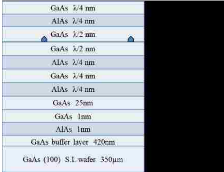
Figure 2.2. Structure diagram of a QDs-in-cavity sample.
