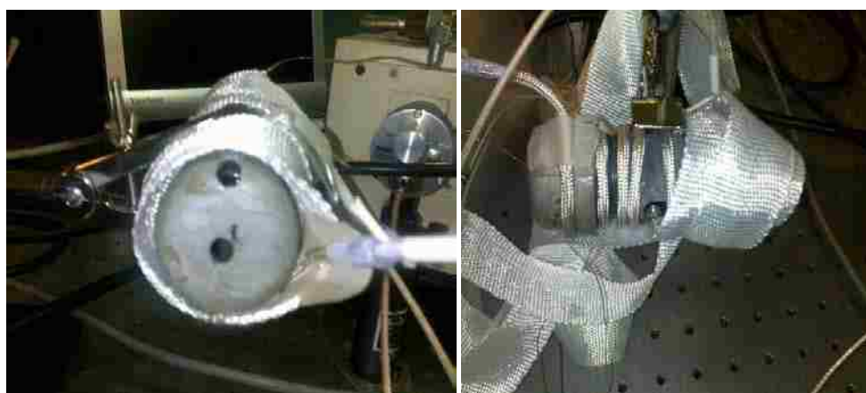
Figure 3.2 (a) side view with both laser beam entrance and observation hole. (b) cell wrapped in metal “oven”, evenly wrapped heater rope, and insulated with fiberglass rope.
