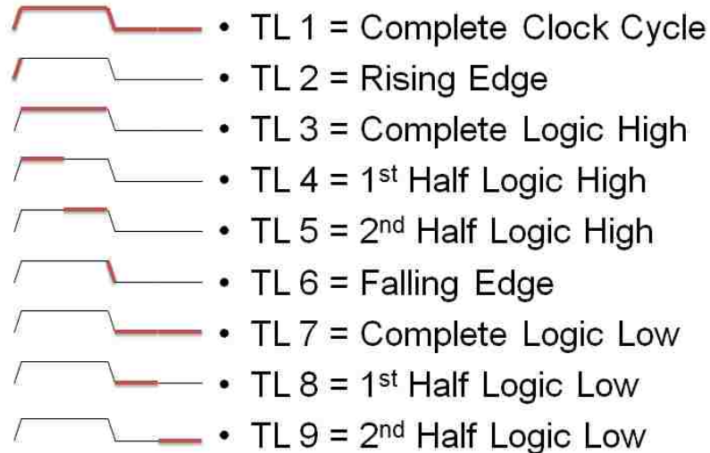
Figure 26. Based on the LP2052 parallel instruction cycle process, 9 different target locations have been defined to be injected with RF.
