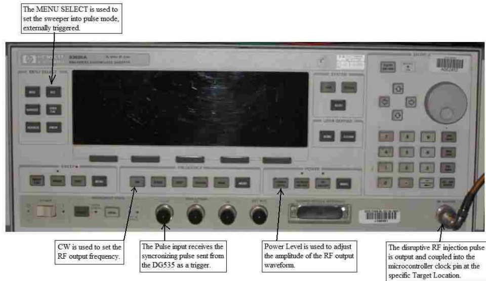
Figure 33. Photograph of the HP 83620A synthesized sweeper used in the experiments.
