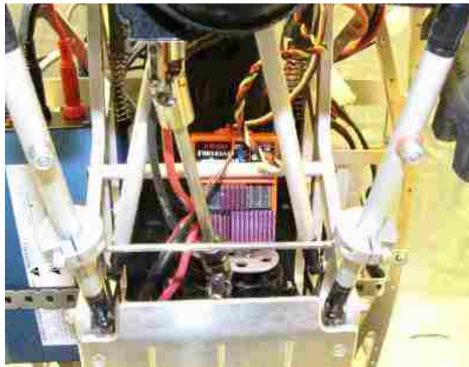
Figure 3.5: The Novak Super Rooster mounting location.
