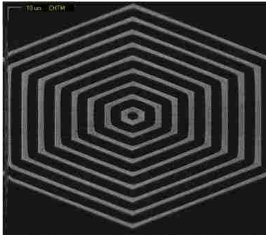
Fig. 4.20 SEM image of a multi-hexagonal annulus pattern is shown. These structures could potentially be threading defect free, but also present us with a large active area, thus leading to a high power threading defect free LED.
