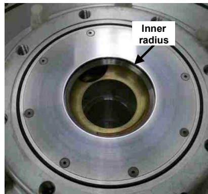
Figure 7.3: Redesigned modulating cavity base plate in the reltron.
