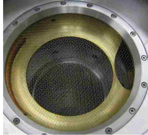
Figure 7.11: New grids in the reltron modulating cavity.
