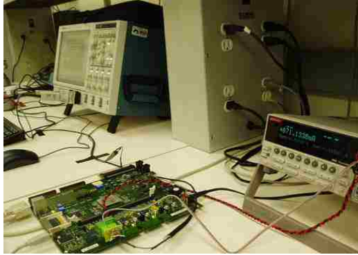
Fig. 5.1: XUP V2-Pro board and experimental setup with Keithley 2400 source meter and Tektronix TDS 7254 digitizing oscilloscope.
