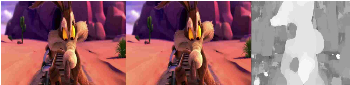
Figure 16. Examples of the binocular stereo image used as an input and the left disparity map obtained after running our algorithm.
