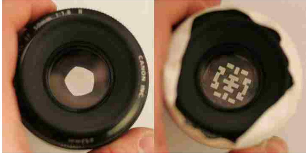
Figure 6. Normal aperture and coded aperture (Levin, et al. 2007)
