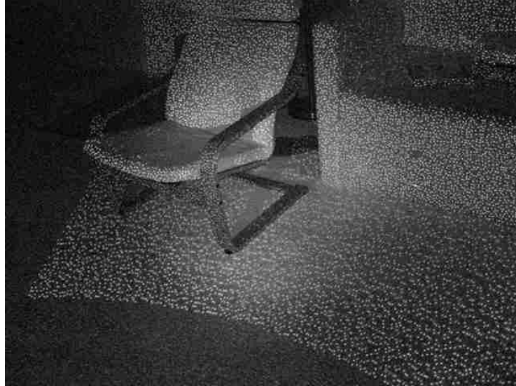
Figure 12. Infrared picture showing the structured light projection.
