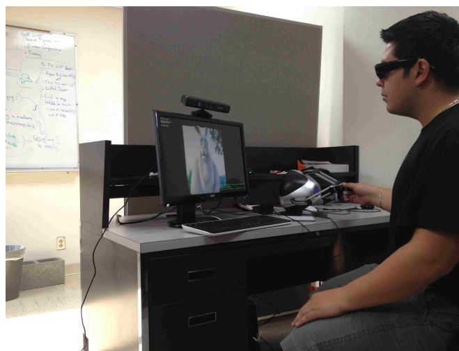
Figure 4. A user using the system. You can see the many hardware parts that conform the system: the Microsoft Kinect on top of the 3D Screen, the user wearing 3D glasses and the Novint Falcon.
