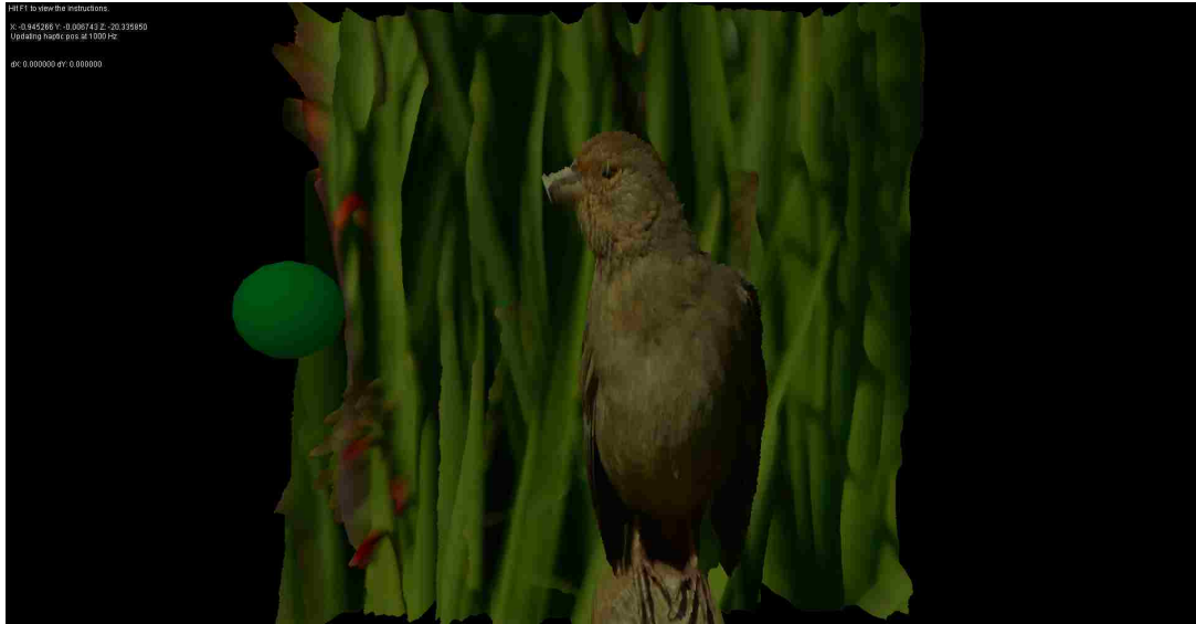
Figure 18. When going with a very high resolution depth map some undesirable effects can appear and can slow down the frame rate.
