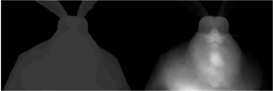
Figure 8. The bunny on the right is the depth map straight from the rendering system, there is little detail that can be rendered in a device with limited resolution. The image on the right is the depth map after being detail mapped; the details can be appreciated with the naked eye.
