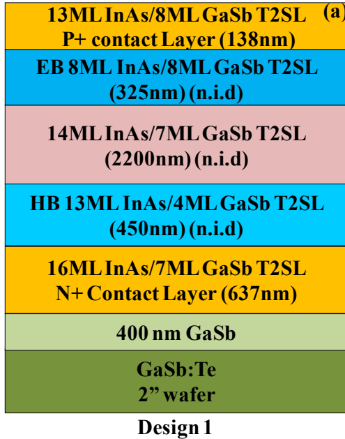
Fig. 5.2. (a) Heterostructure schematic, (b) XRD plot of pBiBn Design 1.
