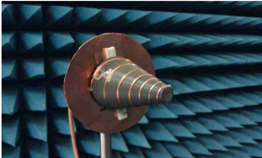
Figure 9.3 Mounted bottom fed CLSA in the anechoic chamber.
