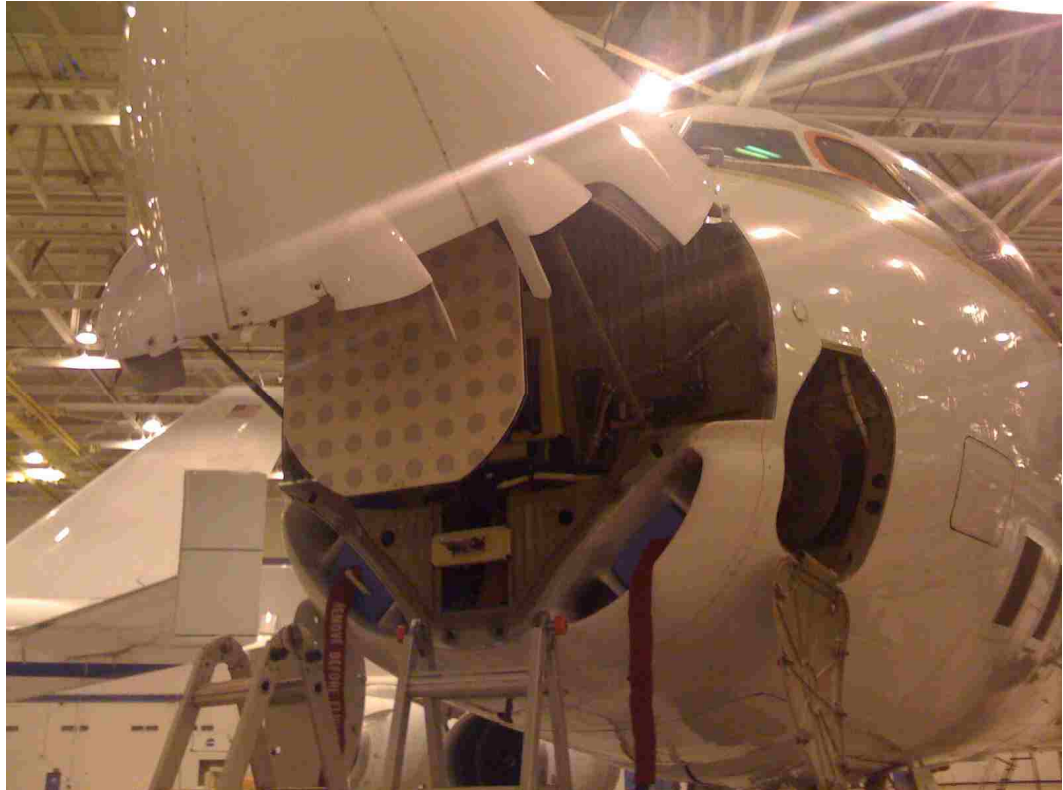
Figure 40: The 34" HSDTA installed and ready for flight aboard a DC-8 aircraft.
