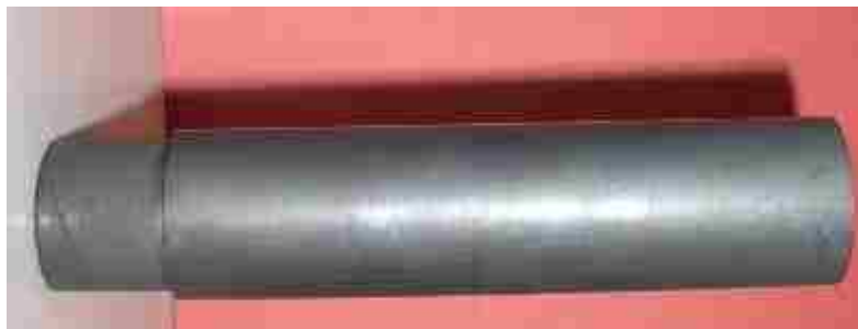
Figure 3.3. Photograph of a solid cathode used in UNM experiments.
