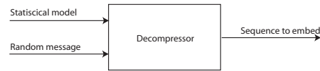
Figure 4.4: The decompressor uses the statistical model of the coverttext to decompress a random message so that the output sequence has the desired statistical properties of the model. The output sequence can then replace the least-significant portion of the coverttext to produce the stegotext.
