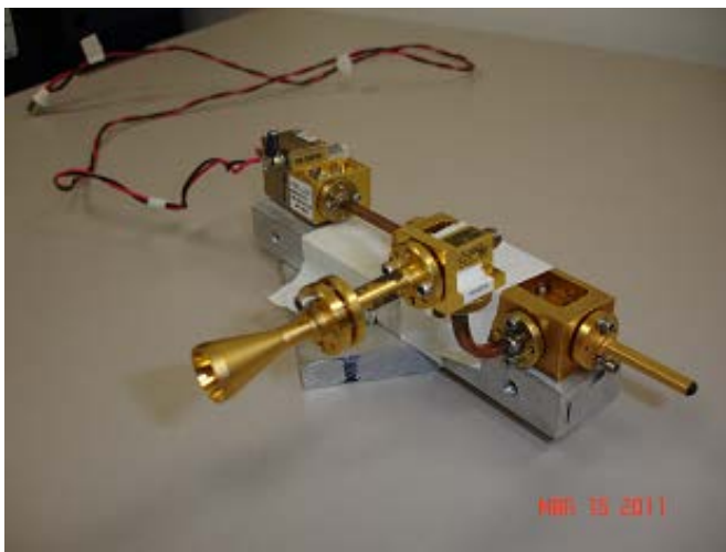
Figure 5-6: Mixer used as a detector after the original detector failed.
