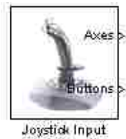
Figure 3.4: The Joystick Input block from MATLAB's Simulink 3D Animation.
