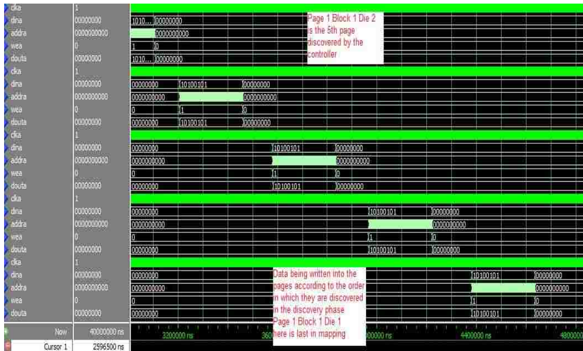
Figure 4.13: Functional Timing Simulation of 3D NAND Flash Controller Data write
