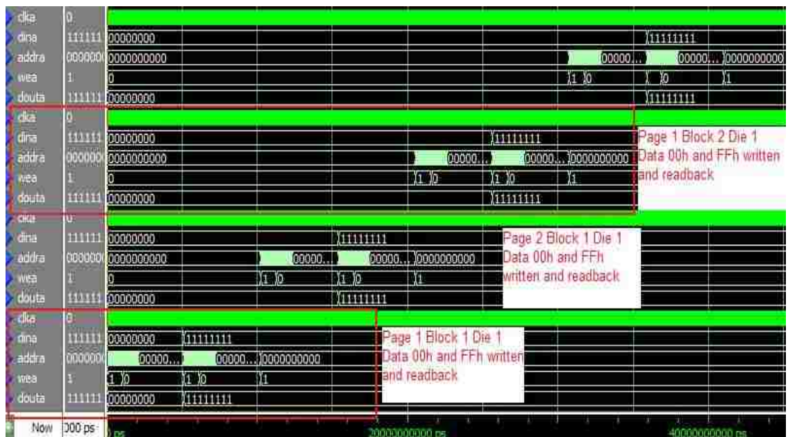
Figure 4.6: Functional Timing Simulation of Boot Unit of 3D NAND Flash Controller
