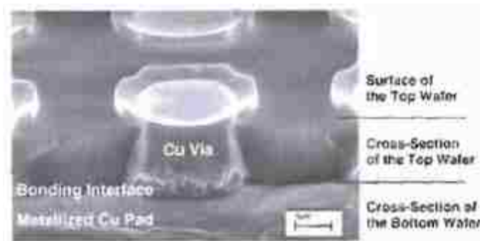
Figure 2.4: A close-up of the cross-sectional SEM image of a Cu via successfully bonded to a Cu pad
