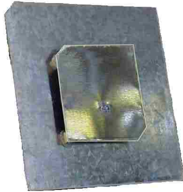
Figure 6.5: Hardware — patch antenna.
