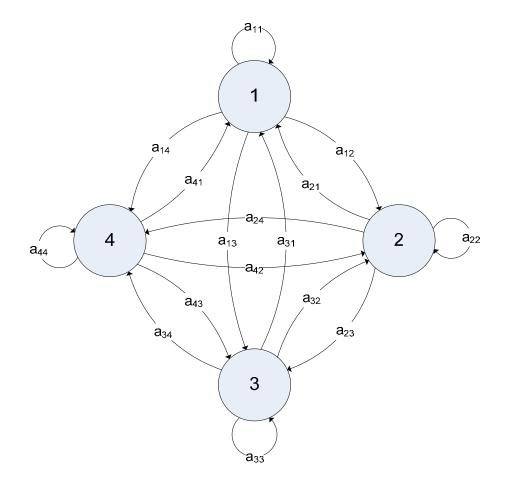
Figure 2.1: 4-state transition diagram
