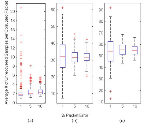
Figure 5.7: Average number of unrecovered samples at different error rates for 12-bit signals. (a) Results with 1 bit error per corrupted packet. (b) Results with 2 bit errors per corrupted packet. (c) Results with 1 bit error per corrupted packet and only decoded in the frontward direction.
