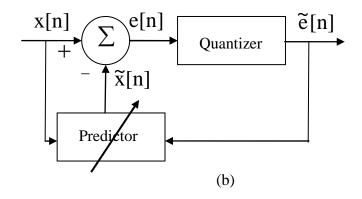
Figure 3.1: (a) DPCM – First order linear prediction model (b) Nth order linear prediction model
