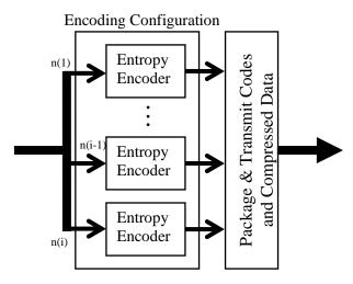
Figure 4.1: Top level diagram of signal encoder where n(0) through n(i) are the bit widths of the data going to the segment encoders, and the sum from n(1) through n(i) equals the bit width of the original ECG signal
