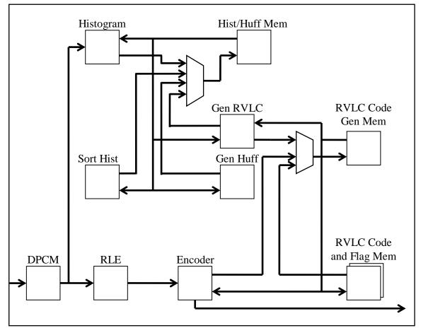
Figure 4.2: Entropy coding system top level view for a 4, 6, or 8-bit segment encoder with the ability update the RVLC tables
