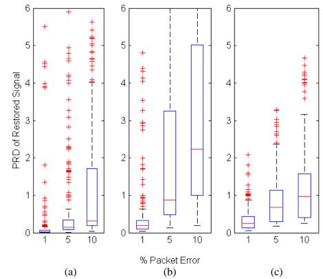
Figure 5.8: Average PRD of restored 12-bit signals with errors introduced. (a) PRD results with 1 bit error per corrupted packet. (b) PRD results with 2 bit errors per corrupted packet. (c) PRD results with 1 bit error per corrupted packet and only decoded in the frontward direction.
