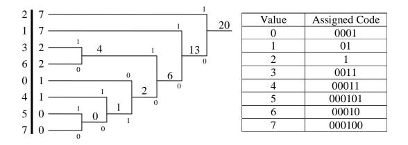
Figure 3.3: Example of Huffman code table calculation using 8 values and 20 total occurrences of those values
