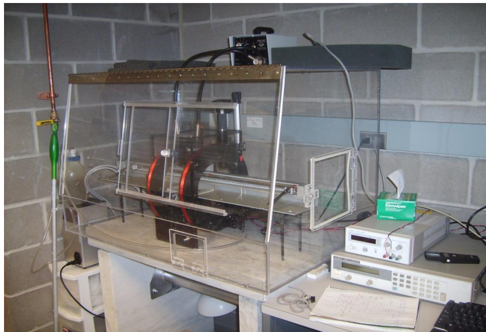
Figure 3-2: The interfacial stress rheometer (ISR) placed on a vibration isolation table inside a home built environmental chamber used to measure the surface shear rheology of interfaces.
