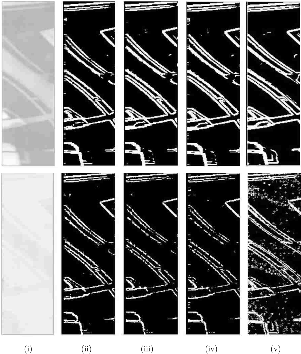
Figure 5.16: Comparison between the SRC with the 2-band min-max signature and the MCG edge detectors for raw (top row) and normalized (bottom row) AHI testing data: (i) AHI test image at band 10; (ii) SRC edges E_{BG} ; (iii) SRC edges E_{RG} ; (iv) combined SRC edge map; (v) MCG edge map.
