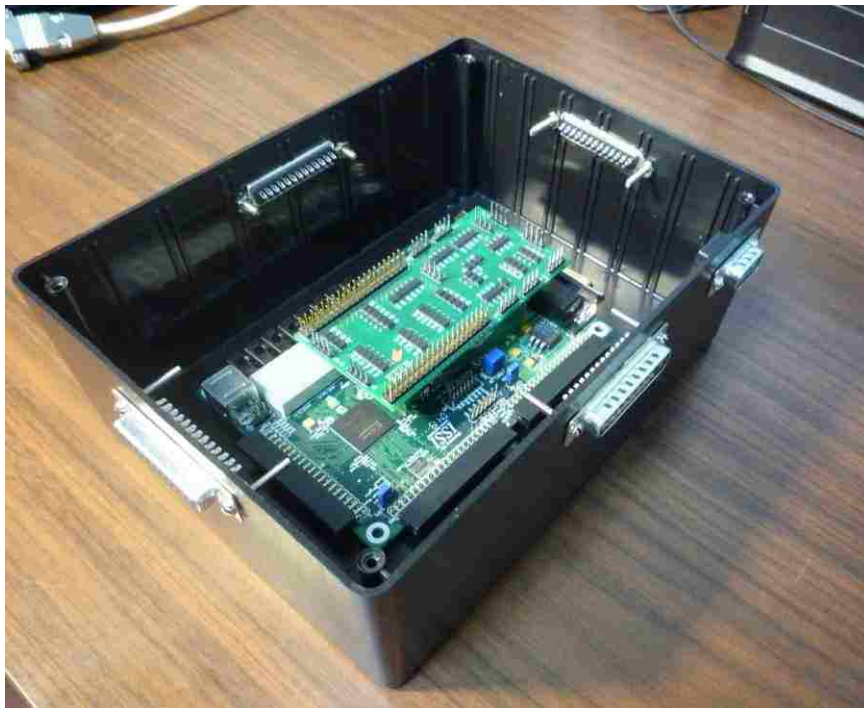
Fig. 15 Initial prototype of one Cell. 25 pin D-sub connectors are used for cell to cell connections. The bottom board layer is a Spartan 3 Board, and middle layer the custom designed relays board.
