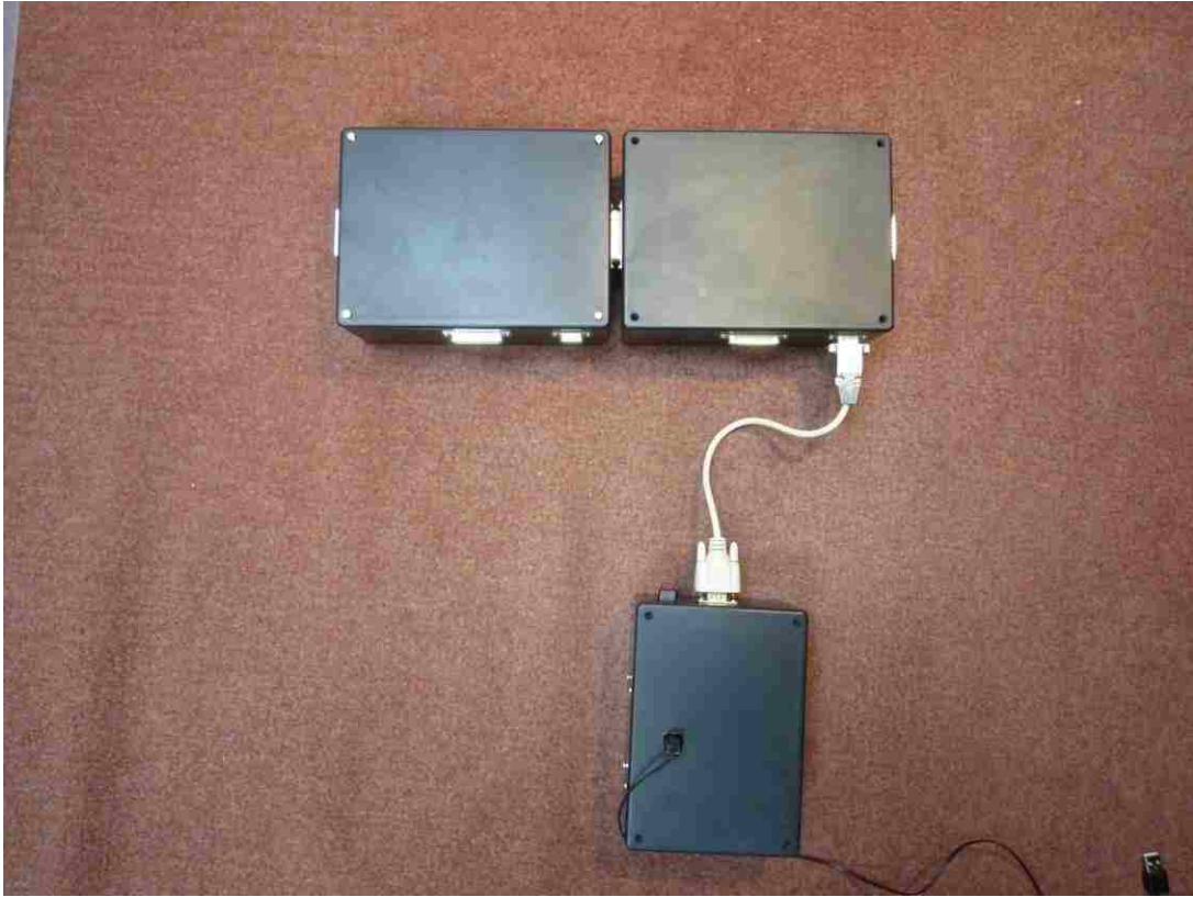
Fig. 16 Example of multiple cells joined together. The bottom enclosure is the communication and power enclosure. The USB connection leads to a laptop which runs the cell management unit.
