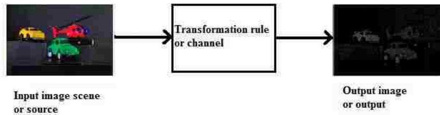
Figure 1.1: Schematic of the PCI system considered in this thesis. The figure shows a source image, the transformation rule and the output image. These components of the PCI system can be identified as source, channel and output of a communication system. In most scenarios of interest, the output image is a sparse, binary array since the photon stream is very weak.
