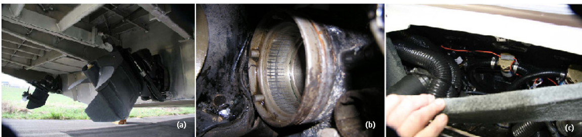
Figure 1. Examples of Watercraft Areas; (a) Category I: Hull; (b) Category II: Gimbal area; (c) Category III: Ballast system.
