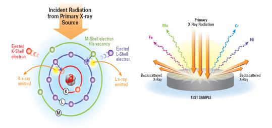
Figure 1. X-Ray Fluorescence Source: (Thermo Scientific-Niton UK, 2003)
