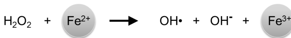
Scheme 1.2 The Fenton reaction leading to production of hydroxyl radical, mediated by Fe(II). This reaction can also take place in the presence of Cu(II).
