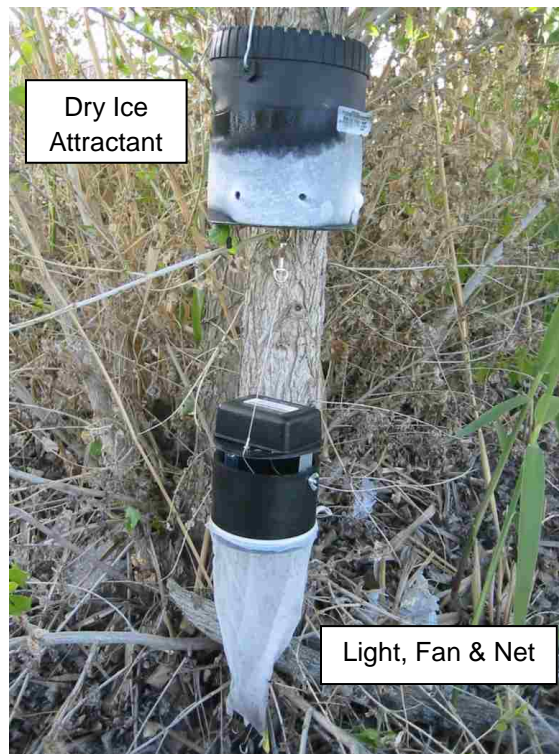
Figure 5. Encephalitis Vector Surveillance Trap. Source: SNHD
