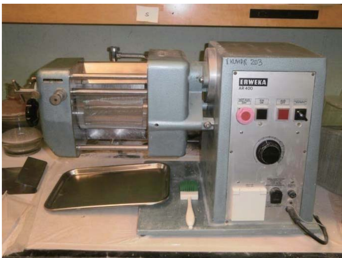
Figure IV-2: Oscillating granulator used as an extruder.
