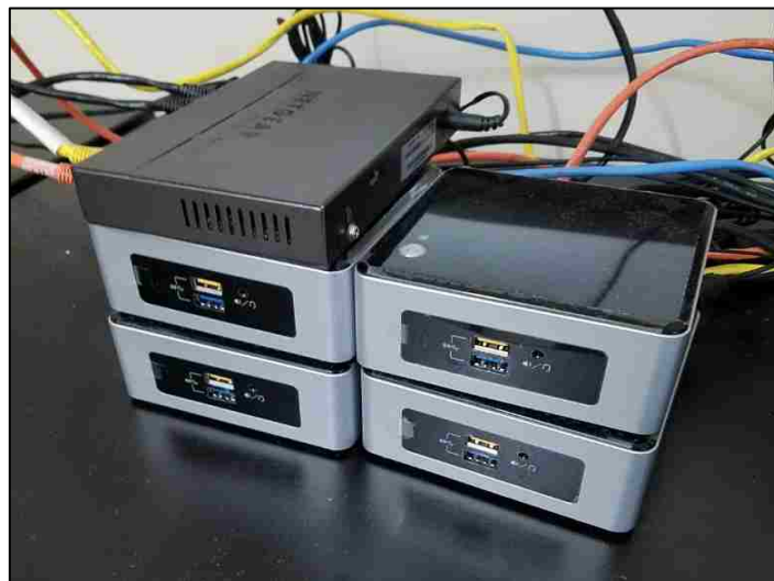
Figure D-1 Hadoop Testbed
