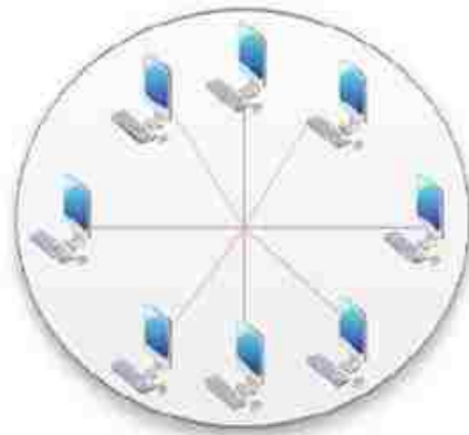
Figure 2: ZigBee Star Topology [21]
