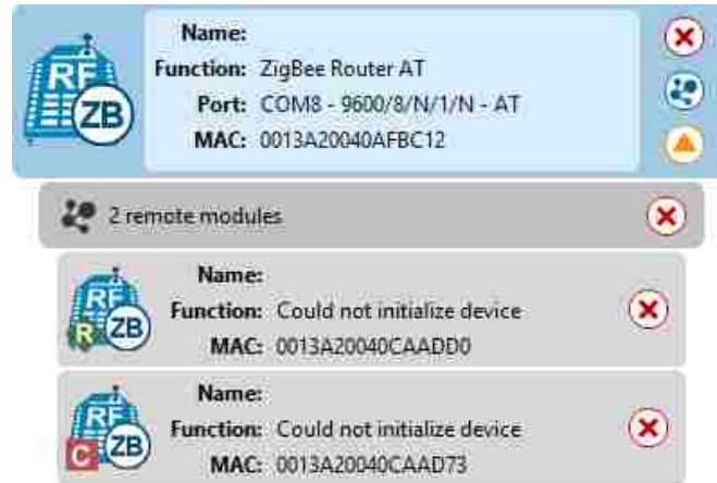
Figure 36: Attacker’s Device Joins the ZigBee Network Setup with Unencrypted Network Key
