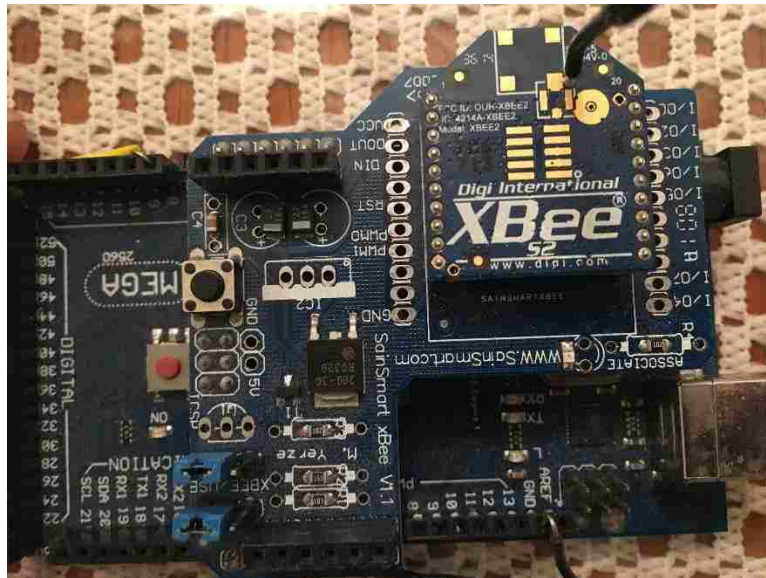
Figure 24: XBee Module Connected to The XBee Shield
