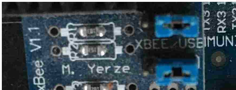
Figure 25: XBee Shield - Jumpers Settings (1)
