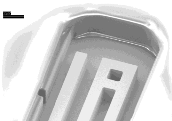
Figure 146: Structures to be free-standing are not encapsulated (such as this electrostatic actuator) while everything else is encapsulated in SU-8.
