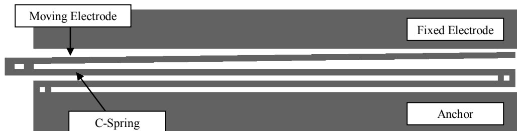
Figure 52: Angled electrostatic clamp which makes use of a small-gap starting zone on the right to reduce the required pull-in voltage.
