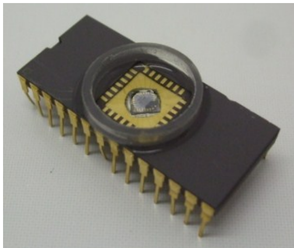
Figure 149: A completed chip with PDMS encapsulation and polypropylene dish.
