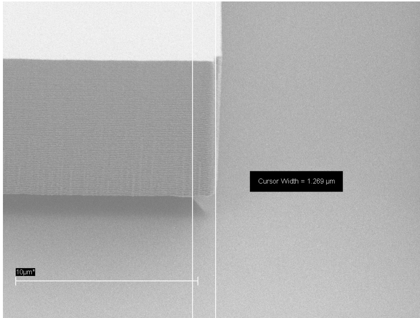
Figure 123: Silicon block after DRIE, metal and oxide pre-etch with 5:1 BHF for 10 min.
