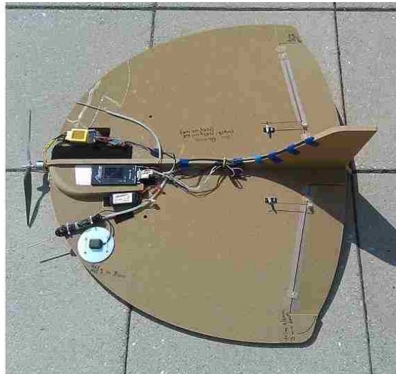
Figure 3.23 – Testing platform used in this work. During testing, the aircraft was flown manually while telemetry data were logged via the on-board Piccolo SL autopilot system.
