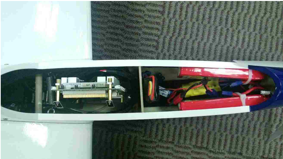
Figure 3.10 – Batteries and autonomy subsystem installed into the Fox fuselage. Pictured here are two 3300mAh batteries, one for powering the motor and actuators, and the other for powering the on-board computer; and a 1350mAh battery for powering the Piccolo autopilot. In alternative configurations, the 1350mAh battery is mounted behind the center of mass.
