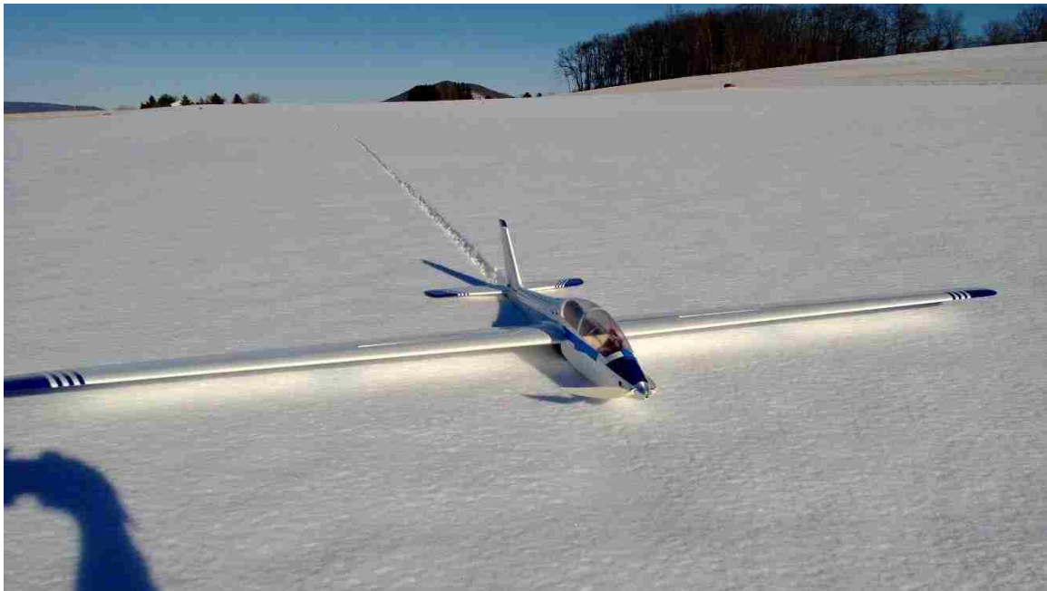
Figure 3.25 – The Fox gliding platform landing in a snow-covered field after a flight test. This particular test was conducted under manual control.
