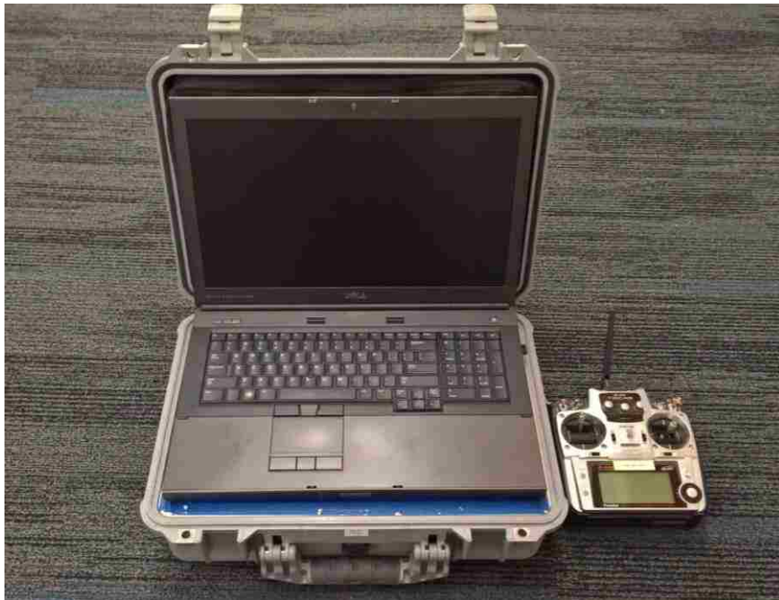
Figure 3.11 – The portable ground station. The ruggedized case contains a radio transceiver that is used to receive telemetry packets from the Piccolo autopilot and send autopilot loop control packets upstream. Telemetry information is monitored on the laptop computer, which connects via serial port to the ground station. The pilot console (pictured) connects to physically to the ground station via a serial link and allows a pilot to take over manual control of the aircraft, bypassing the autopilot.
