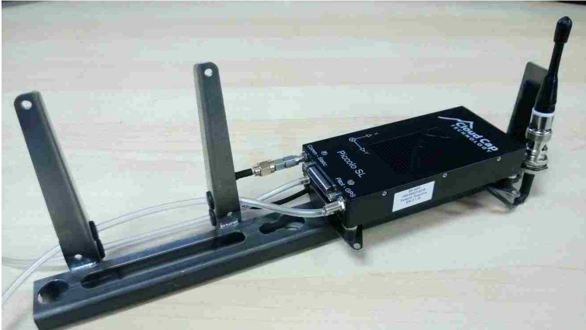
Figure 3.3 – A custom steel chassis for avionics. It is installable in the fuselage of the glide. Pictured here is the Piccolo SL autopilot mounted on rubber standoffs to isolate it from vibrations. The two plastic tubes connect to the static and dynamic portions of the pitot sensing system. The antenna pictured here was a preliminary design that was abandoned in favor of a whip antenna that extends along the fuselage into the vertical stabilizer.
