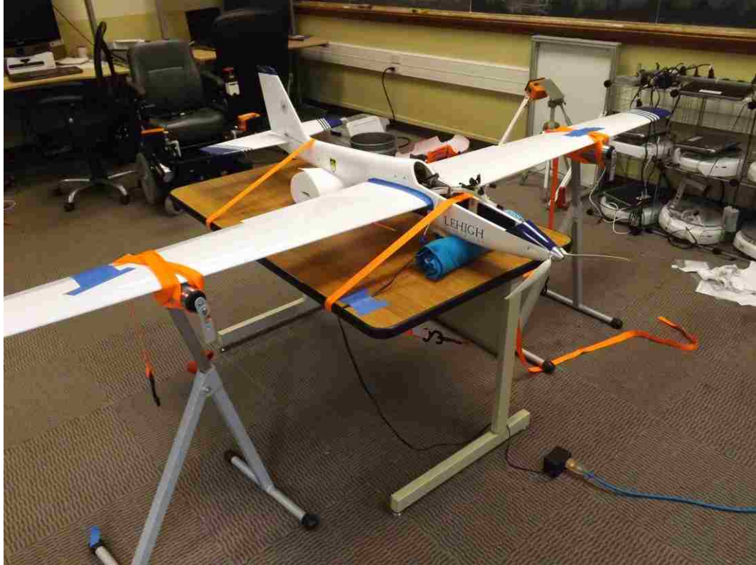
Figure 3.19 – The experimental setup of the vibration test. The fuselage was leveled under two compressible rolls and secured to a table using ratcheting ties. The motor was then run through its operational range and gyroscope data was recorded via the Cloud Cap Command Center logging facility.
