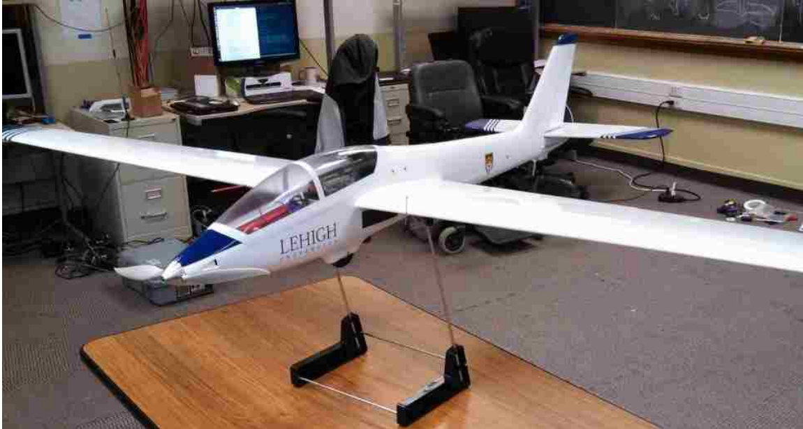
Figure 3.1 – Fox dynamic soaring platform balanced on a center of mass calibration device. The Fox has a wingspan of 2.8 m and an empty mass of 2.90 kg.
