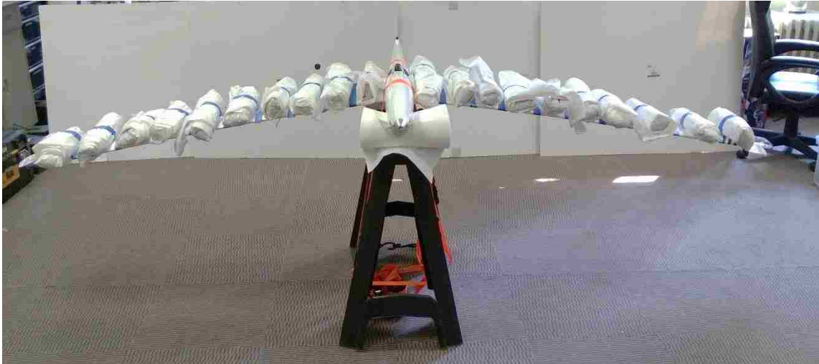
Figure 3.13 – The Fox platform during the wing load test. One-kilogram bags of pea gravel were placed on the wing to simulate a high load turn. The load test was performed for 5 minutes, and then the bags were removed, and the structure was inspected for damage. Preliminary testing revealed damage to the structure of the wings and wing spar.
