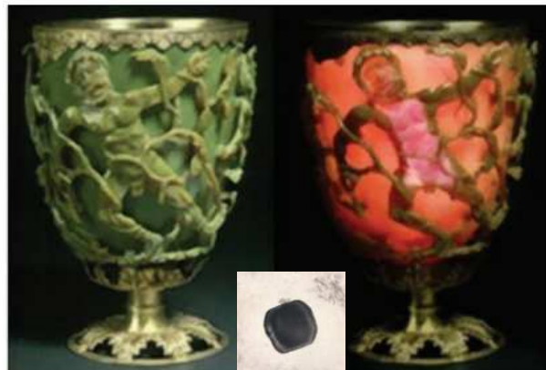
Fig. 1.2 The Lycurgus cup in British Museum dated back to 4th century AD. Due to scattering of metal nanoparticles on sidewall (5–60 nm in diameter), the cup appears green in reflected light, and red in transmission light. Inset: SEM image of a typical nanoparticle embedded in the glass.
