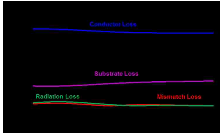
Fig. 4-7 Different losses of shunt MEMS switch. The results were normalized to the total switch loss.
