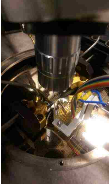
Fig. 3-12 Test setup for characterizing the 3-bit phase shifter using a homemade DC probe-card.
