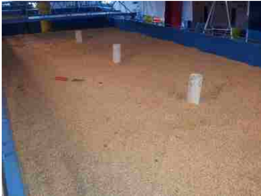
Figure 4.6: Large soil box for simulations of subsurface event detection.
