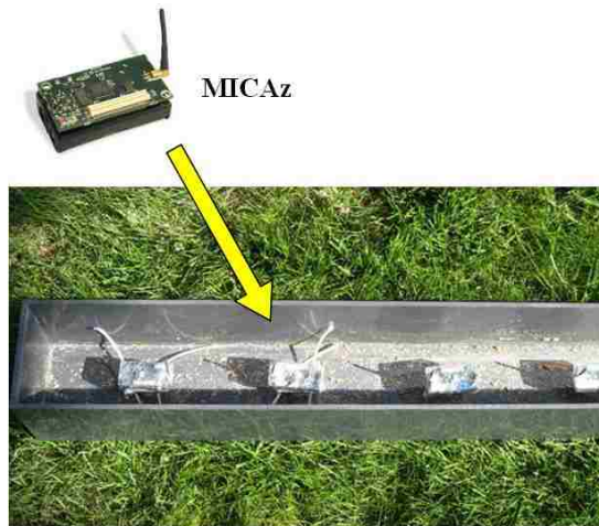
(b) PVC box with sensors before soil filling
