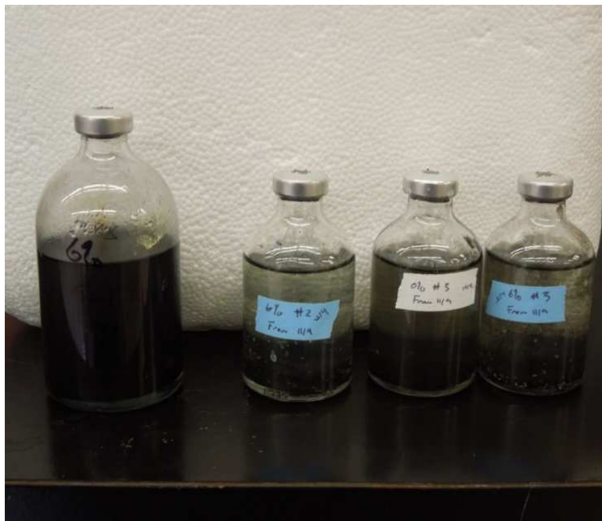
Figure A.1. Enrichment cultures of SRB grown in Postgate Medium C (6.0 g L -1 Sodium lactate, 44.5 g L -1 Na 2 SO 4 , 1.0 g L -1 NH 4 Cl, 1.0 g L -1 Yeast extract, 0.5 g L -1 KH 2 PO 4 , 0.3 g L -1 Sodium citrate·2H 2 O, 0.06 g L -1 CaCl 2 ·6H 2 O, 0.06 g L -1 MgSO 4 ·7H 2 O, 0.004 g L -1 FeSO 4 ·7H 2 O, with a final pH between 7.3 – 7.7). Attempts to isolate pure cultures were unsuccessful.
