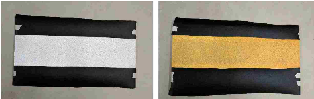
Figure 47: White (left) and yellow (right) roadway marking samples (with glass beads).
