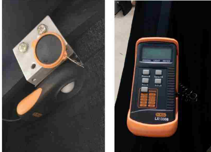
Figure 31: Dr. Meter LX1330B digital illuminance meter receptor (left) and display (right).
