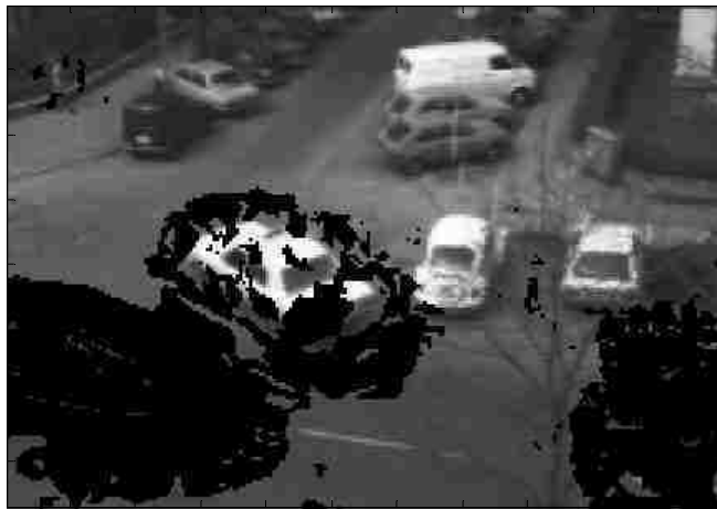
Figure 4.33. Confidence map of the velocity estimates. Dark areas with low confidence are located on the objects with the largest velocities close to 3 pixels per frame.
