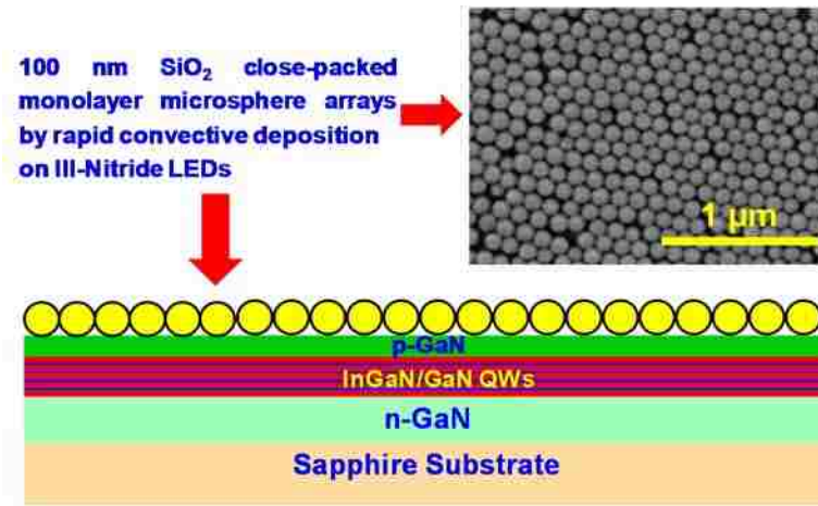
Figure 3-2. Schematic side view of the simulated microsphere LED device, and the corresponding SEM images of 100-nm SiO 2 sphere arrays.
