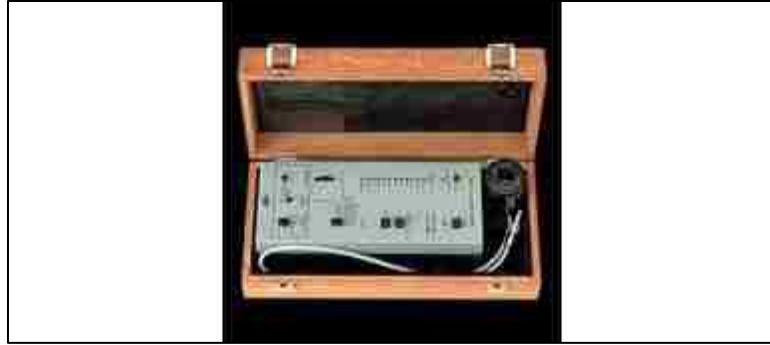
Figure 4.19: Brüel & Kjær Type 4226 Acoustic Calibrator
