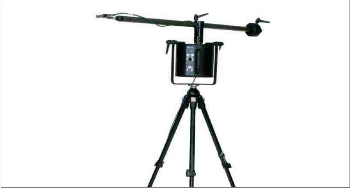
Figure 4.17: Norsonic Nor 265 Microphone Boom
