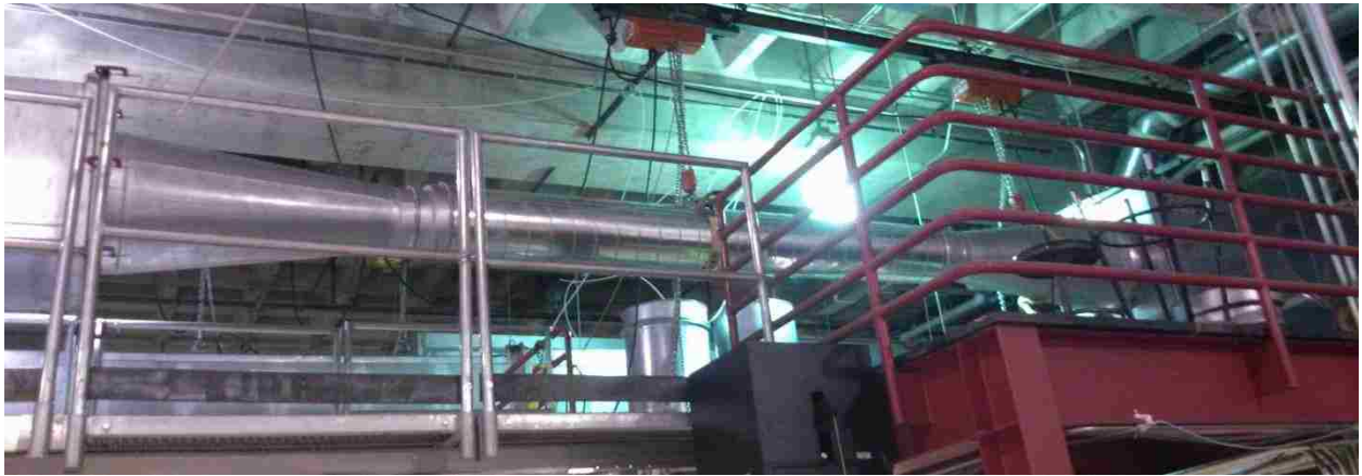
Figure 5.4: 12-in Diameter Duct Test Setup
