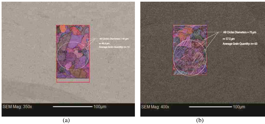
Figure 3.46 EBSD microscopy photos of A36 steel a) non-impact, b) A36 steel impact at 5.80 km/sec Sample locations 6-G.
