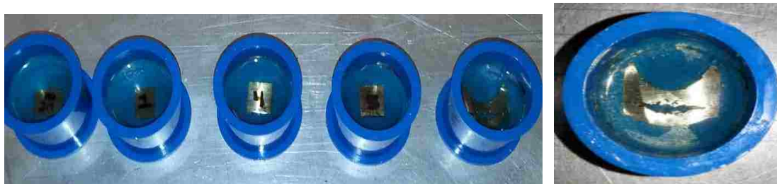
Figure 2.9 Sliced steel specimens in casting molds
