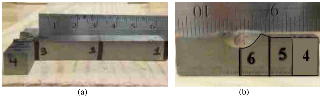
Figure 2.6 Location of six cross-sectional regions used for microstructural analysis
