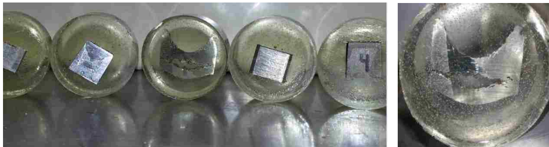
Figure 2.10 Epoxy cylinders with steel slices ready for polishing
