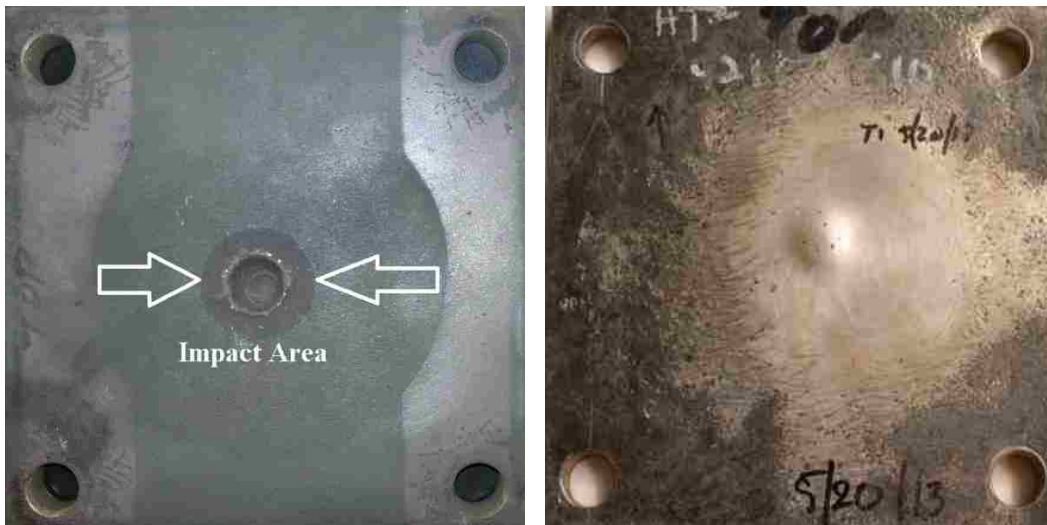
Figure 2.3 front sides (left) and back side (right) visible damage on an A36 steel target
