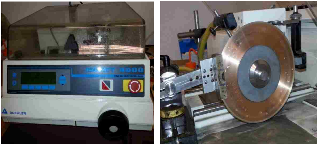
Figure 2.7 Linear Precision Saw (ISOMET 4000) used to slice steel cross-sections
