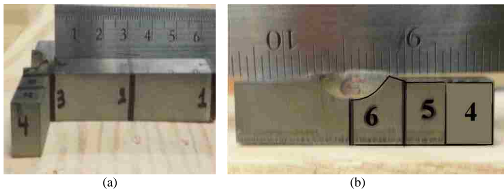
Figure 3.5 EBSD specimen locations were taken from 6 locations along two different lines of a T-shaped specimen of the A36 steel target: (a) Along impact crater perpendicular to impact mid-line and (b) Parallel to mid-line cut.
