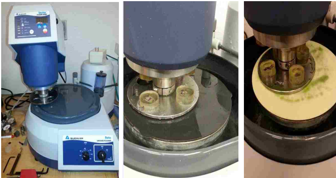
Figure 2.11 Polishing and preparation process of A36, 304L and HY100 steel
