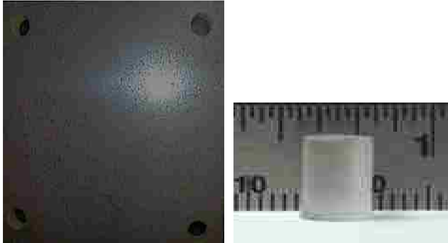
Figure 2.2 A36 target plate before impact and Lexan projectile (not shown to the same scale)
